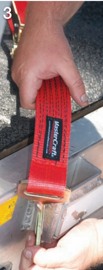
The first step after loading the truck (a C/K in this case) is to secure the ratchet end hook to the trailer.
