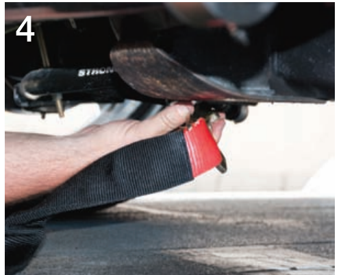
The other end of the strap is hooked to the other side of the control arm mount pocket.
