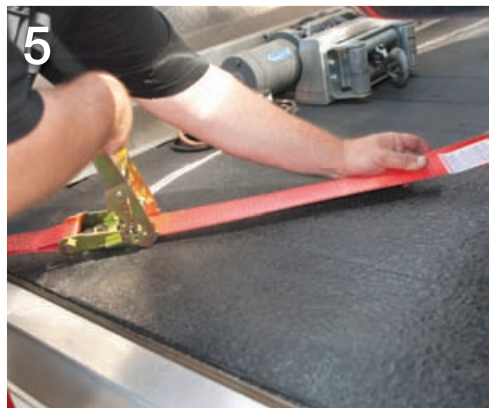
Pull the slack from the strap and crank the ratchet to tighten.
