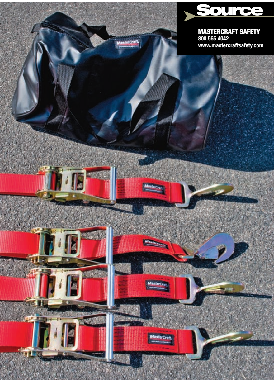
Here are the 8-foot tie downs from MasterCraft Safety complete with carrying bag. The 2-inch wide straps have five sets of stitching for strength. Each strap has a maximum load of 10,000 pounds.
