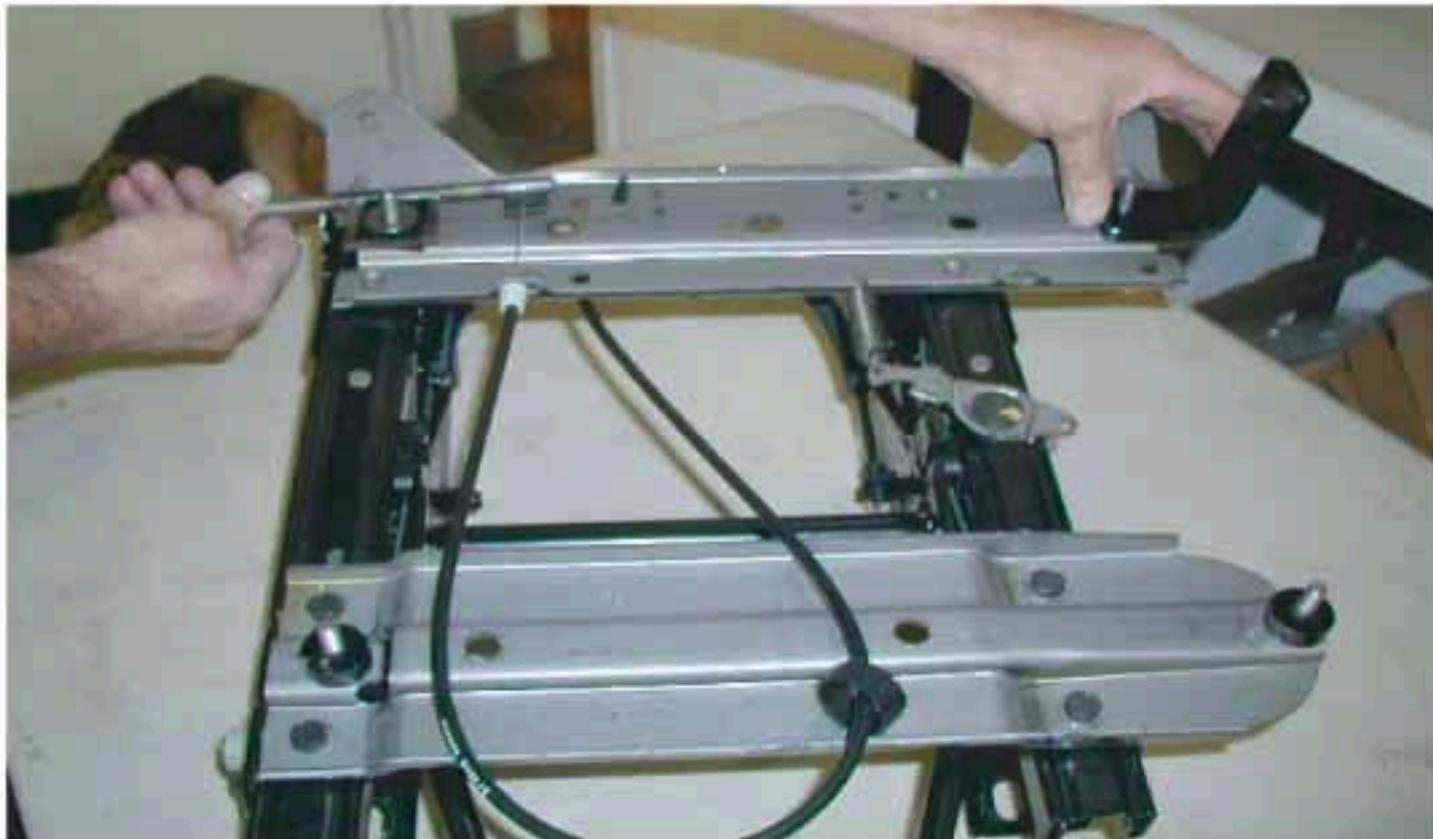
**Step #9** Then mount seat over top of studs using the provided nyloc nuts and washers.
