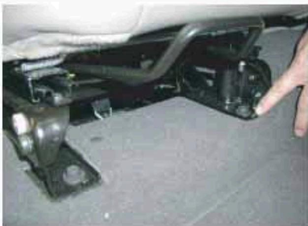
**Step # 2** - Detach the two cables on the inside of the passenger seat. The bottom cable pops off.
