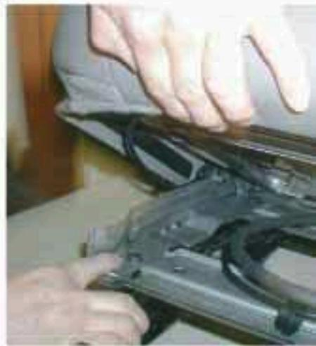
**Step # 6** - Remove the top cable with the black end completely from the riser and discard.
